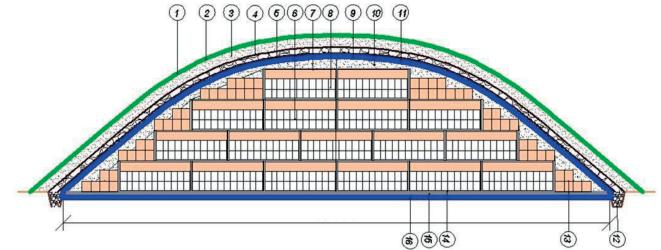
1- grass reinforcement; 2 – natural layer 0,1 m; 3 – natural soil 0,9 m; 4 – quarry stone protection layer 0,5 m; 5 – crushed stone 0,3 m; 6- 20-feet containers with 4 class waste (OHRAW); 7 – contaminated soil; 8 – 4 class waste (OHRAW) in 200l steel barrels; 9 – bentonite mat 2 layers; 10 – levelling layer of sand 0,7 m; 11 - geogrid; 12 – drain trench; 13 – Big Bags with contaminated soil; 14 – reinforced concrete foundation; 15 – crushed stone 0,3 m; 16 – bentonite mat 2 layers
